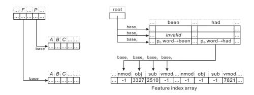
Figure 7: Difference between ordinary base array (left) and base array for 2D Trie (right)
