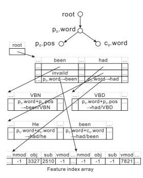
Figure 6: 2D trie for a general template tree. Dashed boxes are keys of columns, which are not stored in the structure
