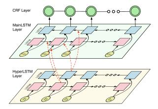
Figure 4: Main architecture of Model-II. We use a HyperLSTM to dynamically generate the weights for the MainLSTM. The HyperLSTM takes feature vectors  $\mathbf{t}$  as inputs, while the MainLSTM takes embedding vectors  $\mathbf{e}_x$  as inputs.
