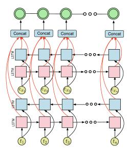
Figure 3: Main architecture of Model-I. The  $\mathbf{e}_x$  and  $\mathbf{t}$  represent character embeddings and feature vectors. The two parallel Bi-LSTMs are used to extract context information and potential word boundary information.
